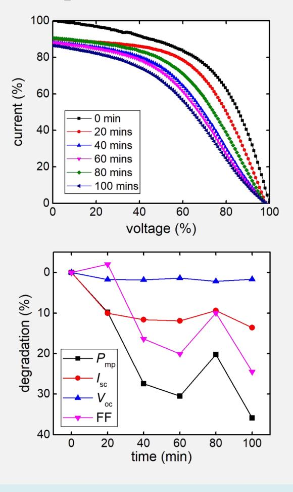
IV curves and cell parameters of an unencapsulated PSK cell are measured after various degradation times at 65 °C in air and 35% humidity.
