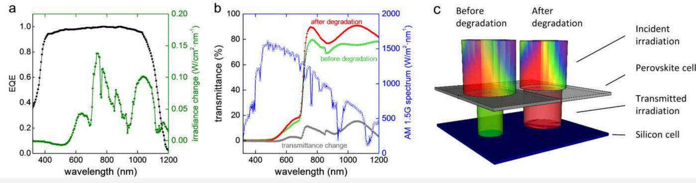
Optical degradation of the perovskite top cell may translate into *Isc* increase at the silicon bottom cell. Based on our in-house fabricated cell, we obtained a ratio of 0.89 between the *l*sc loss at the top cell and the *l*sc gain at the bottom cell.
