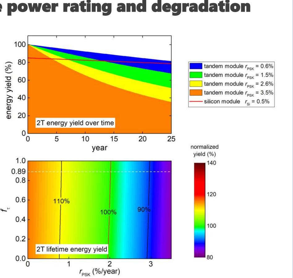
Silicon based perovskite tandem cells have great potential to further improve solar module efficiency. However the uncertainty of perovskite solar cells' long term stability leads to uncertainty of economic competitiveness against conventional silicon modules.
